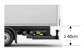
Minimum sensor fitment height must not be less than 40cm from the ground. This prevents giving false detections caused by detecting the ground.
